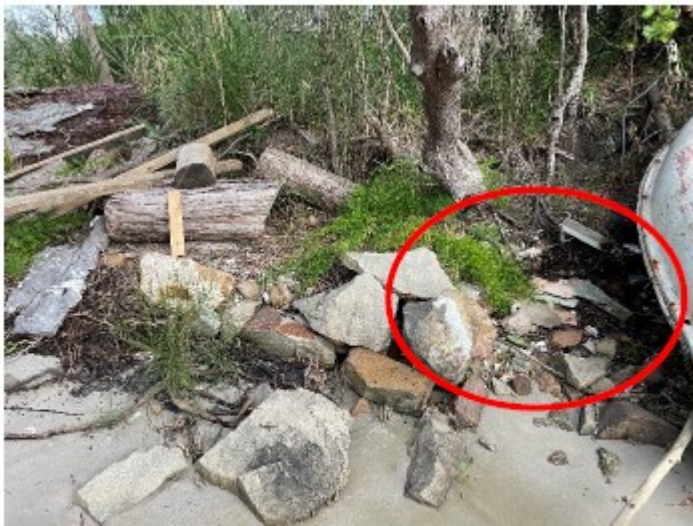
Fibre cement sheeting that may contain asbestos near D5, Ch 180m
